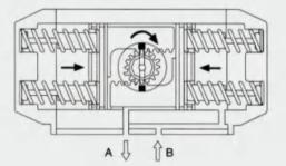
When loss air pressure or power, the stored energy in the springs forces the pitons inwards, causing the pinion turns clockwise while air be exhausted from Port
