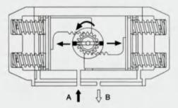
Input the air into Port A forces the pistons move outwards, the pinion turns counterclockwise and open the valve, then the air be exhausted from Port B.
