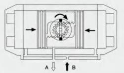
Input the air into Port B forces the pistons move inwards, the pinion turns clockwise and close the valve, then the air be exhausted from Port A.
